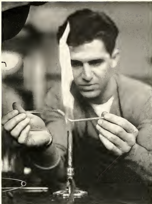
A student uses a Bunsen burner to soften and bend glass. Equipment in labs is kept up-to-date.
