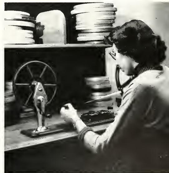
INSPECTING FILM FOR damage, student assistant Janette White works at the splicer, a mechanism designed to join shorter lengths of film. Audio Visual Aids supplies films for all University classes.
